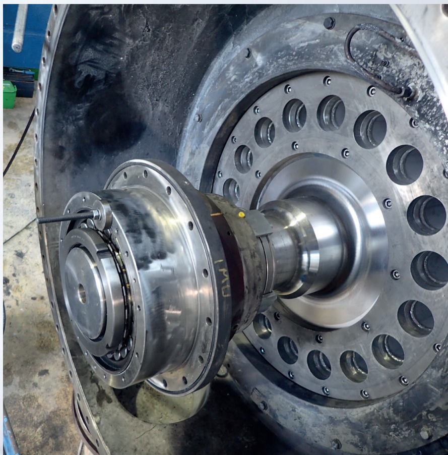
Pre-assembly of the bearing including mechanical seal
