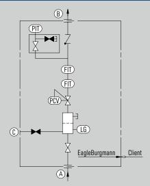
**P&ID for GSS6001-A4 Gas supply system** A Gas IN B Gas OUT
